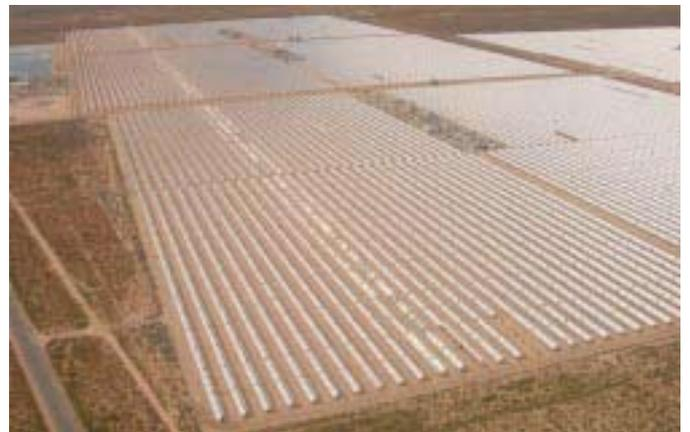
DII uses carefully positioned mirrors in the Sahara desert to boil water and activate turbines. According to the Desertec Foundation,
